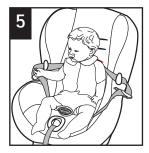
Place the child's bottom and back flat against the child restraint. This will increase comfort and allow the harness to properly tighten.
